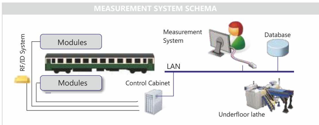
Optionally, identification of the individual cars is possible after mounting of RF/ID tags on them - this way all measurement results can be assigned to individual wheels for further analysis and reporting.
