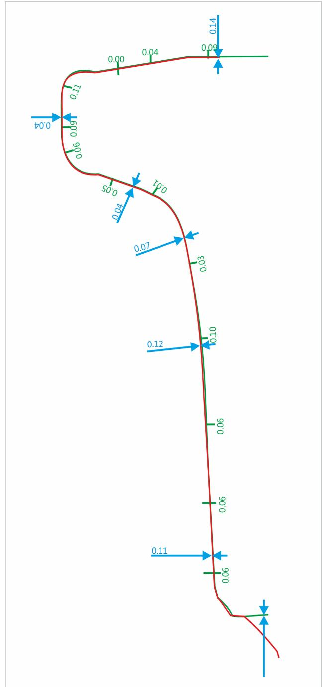
Laser wheel measurement system: repeatability of six wheel optical measurements and difference between them and measurement results obtained with the portable devices.
