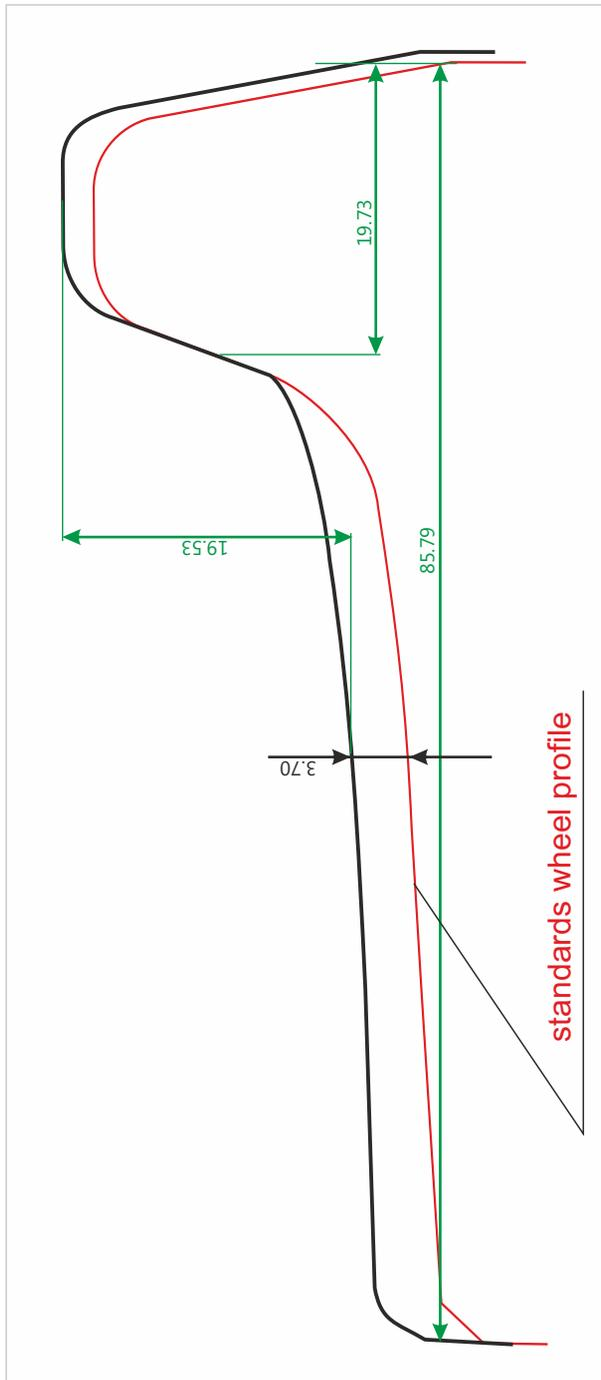
Comparison of the optical measurement results for the tram wheel with measurements obtained using the contact method.
